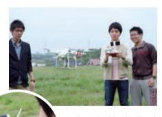
In the study of the situation of contamination in areas affected by the nuclear accident at Fukushima Nuclear Power Station, drones were used to take more refined measurements than measurements taken by people on foot or aircraft. A high-resolution three-dimensional map was created.
